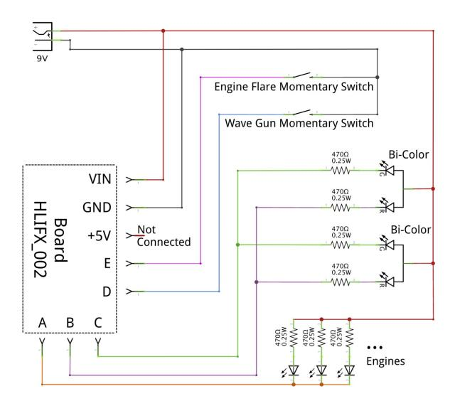
As seen in the schematic above, which color you decide to use for the ramp will tie back to point **B** of the board. Which color you decide to flash will tie back to point **C** of the board. If you decide to connect up bi-color LEDs in this way, then you can have a MAXIMUM of 12 bi-color LEDs connected to the Yamato board, making sure that each color pin is properly resistored for the voltage you are using, as discussed in Section 2.
